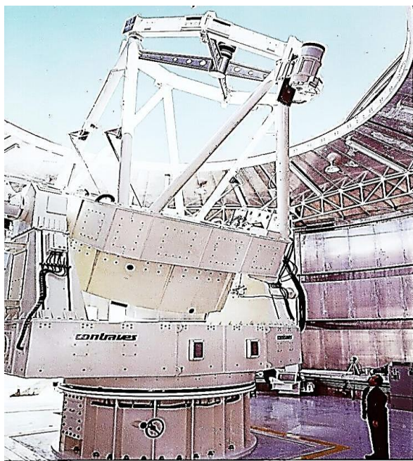
Air Force Research Laboratory Directed Energy Directorate's Starfire Optical Range 3.5-meter telescope. The world-class adaptive optics telescope is the second largest telescope in the Department of Defense.
